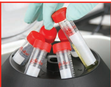
Six position rotor accommodates 15mL centrifuge tubes
